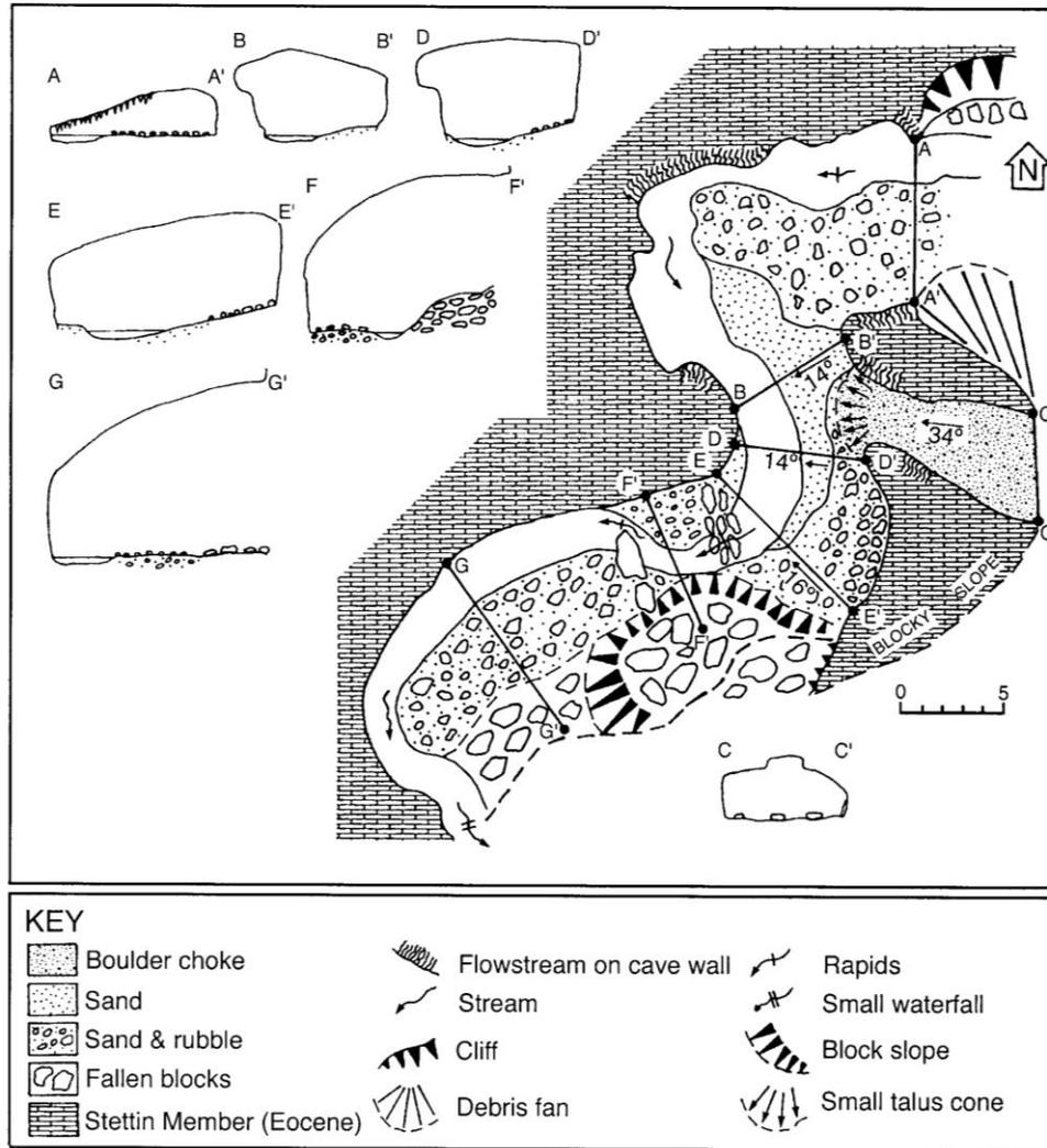
**Figure 5.** Cave survey and selected passage cross-sections (A-A' to G-G') of Wait-a-Bit Cave, parish of Trelawny (after Miller and Donovan, 1996, text-fig. 2). The thick dashed line to the west of E', and south of F' and G', marks the edge of the limestone overhang from the northwest.
